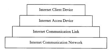
A typical hardware connection for accessing the Internet is shown below. Intercontinental networks include communication backbone. Backbones are typically fiber optic trunk lines. The trunk line has multiple fiber optic cables combined together to increase the capacity.
